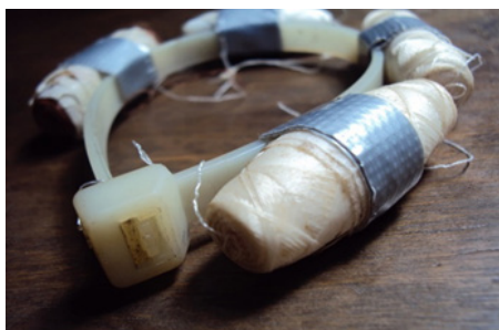
Figure 5 Spool collars that were used to tag cats for tracking at the sampling site Calayan Island, Cagayan Valley, Philippines
